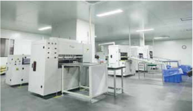
高效过滤器折纸机High efficiency filter origami machine
